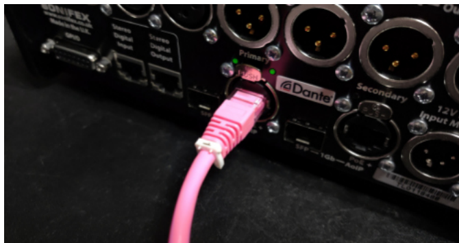
1. Plug an Ethernet cable into the primary port of the AVN-CU2/AVN-CU4.
