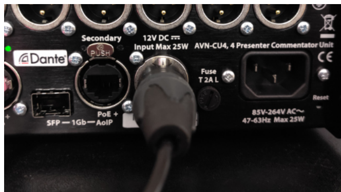
4. If your switch does not support PoE, the DC adaptor can be used instead and has the following pinout: Pin 1: Ground, Pin 2: N/C, Pin 3: N/C, Pin 4: +12V
