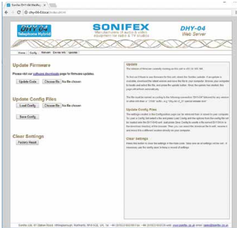
Figure 6-12: Updates Page – to update the system firmware and load/save configuration files.
