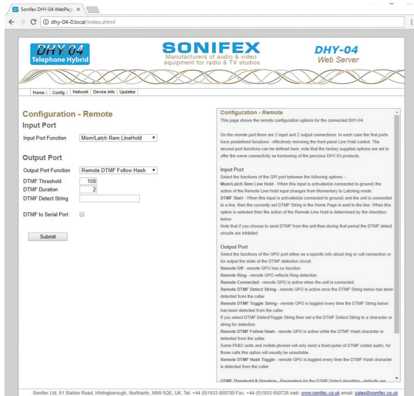
Figure 6-7: Remote Port Configuration – settings of remote port and DTMF detection – accessed via Config Menu drop-down.
